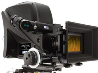
A specialized 4K camera which shoots 'uncompressed' files. Requires a lot of storage on set. Good for critical effects work because the files are not compressed.
