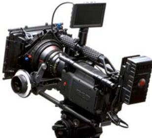
A 4K, high resolution digital cinema camera. Records raw files. A good multi-purpose camera much like a 35mm camera. Uses 35mm lenses and standard accessories.
